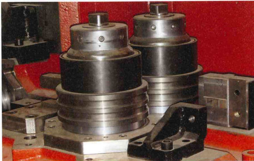
Figure 2. Traditional locking system for the rings of a wire rod block
